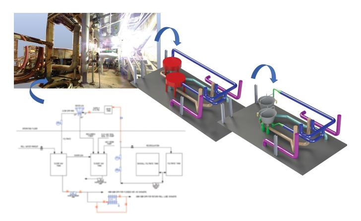
Preliminary engineering for a customer in the south of USA, replacing two old gravity filter concerning finer filtration, energy savings, and reliability
