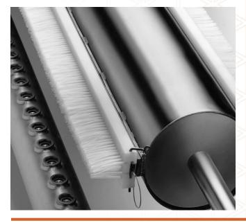
As the fabric passes over one of the brush assemblies, contamination is collected in the bristles. When the brush is fully saturated, the entire assembly is rotated to place a clean brush in contact with the fabric surface. The contaminated brush is then cleaned and conditioned by the stationary or brush shower. The reconditioned brush assembly is now ready for reapplication to the fabric. Rotation can be activated by the handwheel, the solid state control panel timer, or through the mill DCS.
