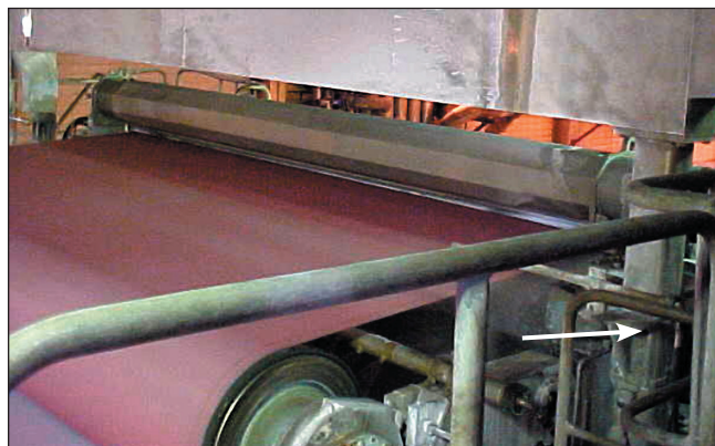
207" (5.25 m) fabric at 3600 fpm (1100 mpm) and 350 psi (25 bar) shower.
