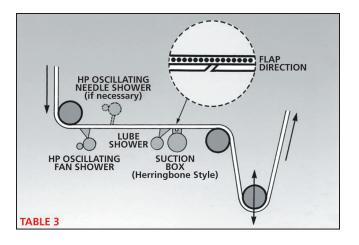
Too often, factors in terms of cfm per square inch of felt suction pipe open area are used to determine vacuum requirements. This is not accurate because the vacuum pump capacity and dewatering assembly must be designed based on the press fabric permeability, the fabric weight, the amount of water applied by the showers, and the machine speed.
