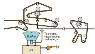
Effluent from press save-all pans, guard board trays, and felt cleaning equipment is heavily contaminated with felt hairs. The RotoFlex resource recovery strainer is captures felt hairs for efficient reuse of press section water.
