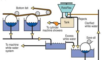
Clarified white water from a cylinder machine save-all generally can not be reused without additional treatment. A RotoFlex resource recovery strainer will remove suspended solids that would blind the coarse bottom felts and plug shower nozzles.
