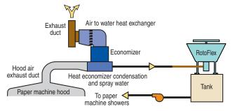
Heat economizers recover heat from the dryer hood air exhaust. In the process, they release a considerable amount of condensation in addition to the cold water that has been sprayed into the air stream to drop the humid air temperature below the dew point. Paper dust and scale contaminate this water. A RotoFlex resource recovery strainer will remove these contaminants permitting this preheated water to be used in the paper machine showers.
