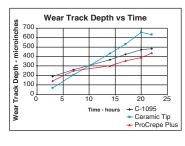
The wearing edge of the ProCrepe Plus Creping blade is resistant to wear but only marginally harder than standard steel. This is why ProCrepe Plus creping blades wear the cylinder less than ceramic and provides longer life than standard steel.
