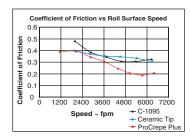
The contact area and shelf of the ProCrepe Plus creping blade wear at a slower rate than steel. This enables the ProCrepe Plus creping blade to be used to produce a higher more consistent quality sheet for a longer period of time.
