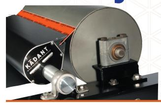
The VeriKleen roll cleaner assembly provides a new, costeffective technology for various industrial applications. Many roll and belt cleaning applications require a design that is both compact and provides excellent cleaning results to improve uptime and reduce maintenance costs.
