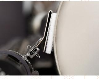
The patent pending VeriLite roll cleaner assembly provides a compact and unique scraper that offers excellent cleaning results to improve uptime and reduce maintenance costs in a variety of industrial roll and belt cleaning applications.
