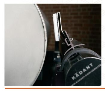
Doctor blades are used to remove contaminants and other matter from roll surfaces. Over time, the build-up on the roll surface requires additional cleaning to provide more uniform roll surface conditions.
