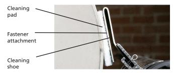
The device is compact and easy to handle. Any pad material can be used by simply adhering it to the fastener on the EzKleen V roll polisher shoe.
