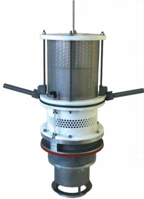
Precise vacuum control is essential for consistent dewatering and formation. The V1000 vacuum control valve automatically maintains vacuum at a specified set-point, despite continually changing stock freeness and vacuum supply levels, due to the force balance control principle.
