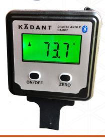
The AngleSet gauge is used to set the proper angle for doctor, roll cleaning, and scraper blades for improved performance and extended blade life. Using the correct blade angle can optimize the life of the roll. The newest version of the AngleSet gauge is Bluetooth capable allowing users to record measurements directly to their mobile device using an exclusive Kadant app.
